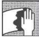
remove any rust if required, sand surface, clean surface carefully with SprayMax<sup>®</sup> Wax&Grease Remover product no. 3680 094; area must be free from grease, dust and humidity. Shake aerosol vigorously for 2 min, spray to test.
